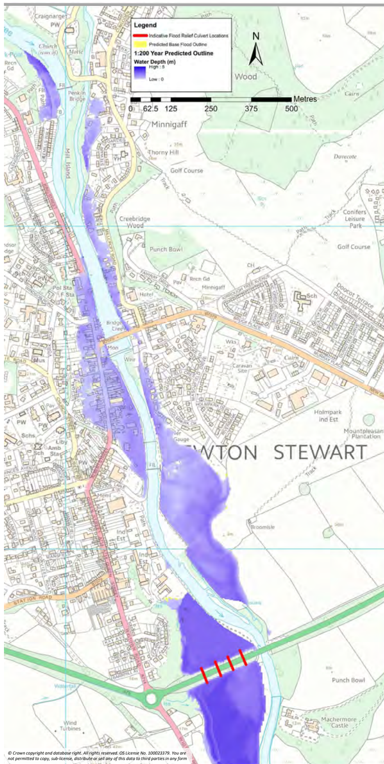
Figure 15-2: 1:200 Year Predicted Flood Outline – Increase A75 Flood Relief Culvert Capacity
