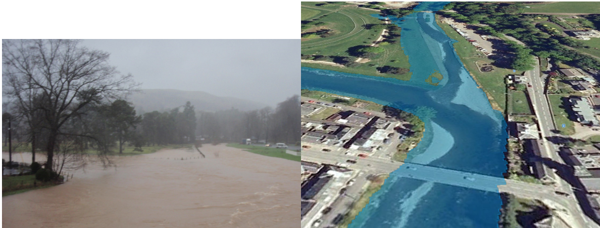
Figure 3.3 Left: Photo taken at 14.10 from Thomas Telford Bridge in Langholm on 05/12/15 Right: Model output at corresponding time superimposed onto Google Earth
