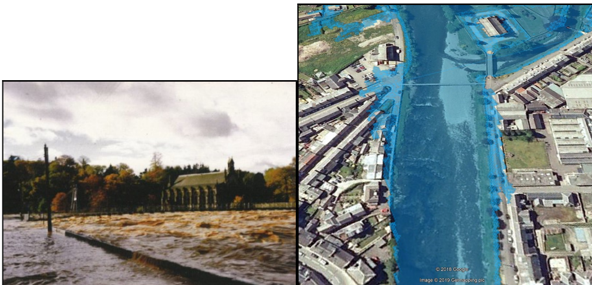
Figure 3.7 Looking downstream from George Street. Left: Photo taken on 31/10/77. Right: 1 in 21 year model output superimposed onto Google Earth
