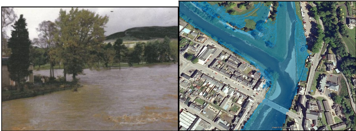
Figure 3.6 Looking upstream from Thomas Telford Bridge. Left: Photo taken on 31/10/77 Right: 1 in 21 year model output superimposed onto Google Earth
