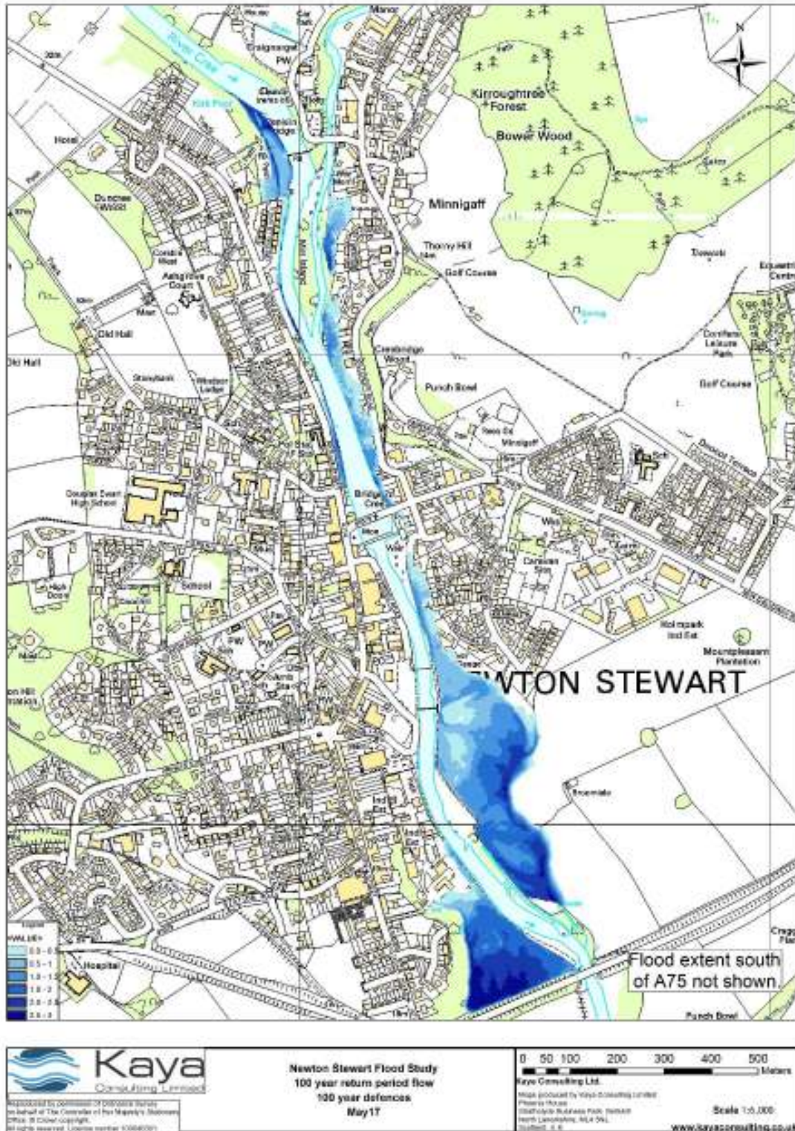
Figure 6: Predicted flood extent for 100 year flood with proposed defences in place
