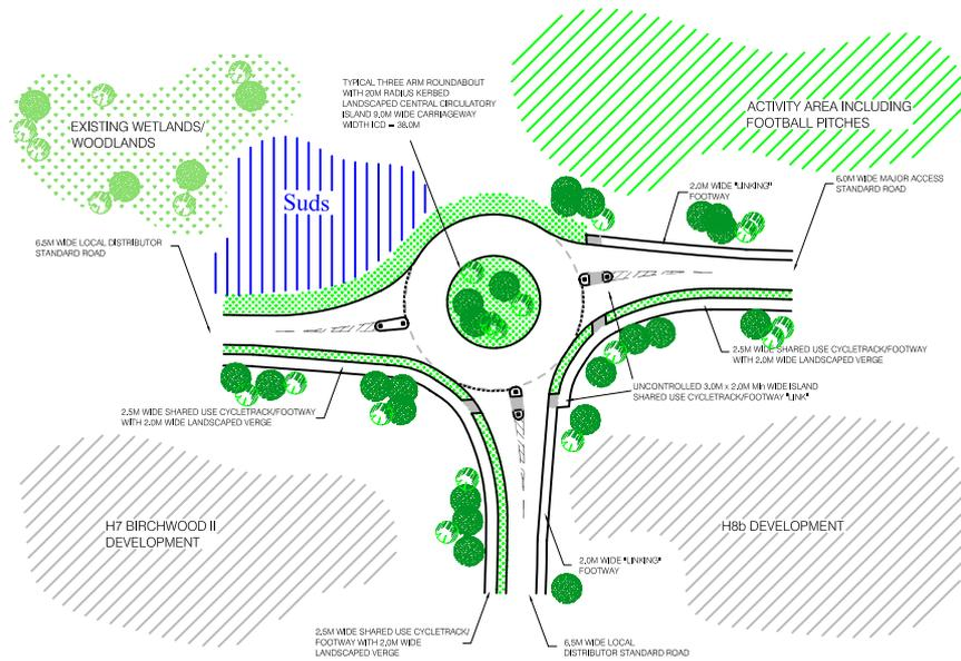
TYPICAL "NORMAL" ROUNDABOUT- TO BE USED ON SOUTHERN DISTRIBUTOR JUNCTIONS
