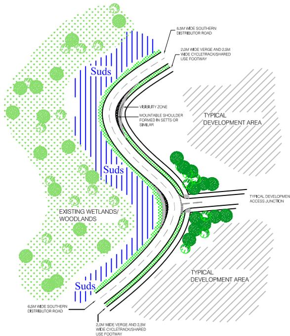
TYPICAL SOUTHERN DISTRIBUTOR ROAD LAYOUT WITH SPEED REDUCING CORNERS, CYCLETRACK/COMBINED FOOTWAY AND DEVELOPMENT AREA ACCESS
