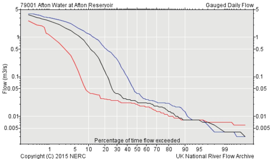
Figure 2-7: Afton Water daily min/max flows over 1965 - 1981 record (courtesy of CEH<sup>11</sup>)
