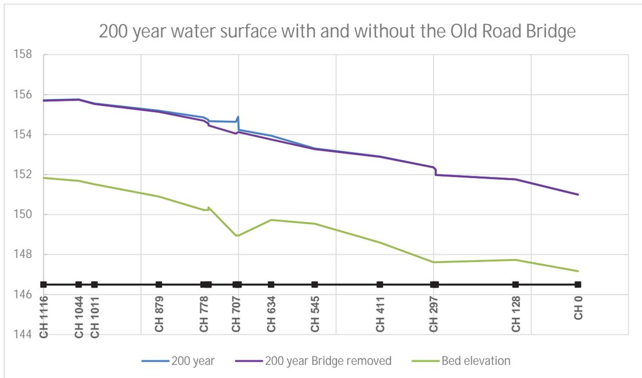
Table 6-2 shows the difference in water surface level (m) for the 25 to 200 year return period for the area of greatest reduction in water surface level due to the bridge removal. The complete set of data with its effect on the Polbower burn is available in Appendix G. This option assumes the Old Road Bridge is replaced at a level with the 200 year plus climate water surface level and has therefore been removed from the model.
