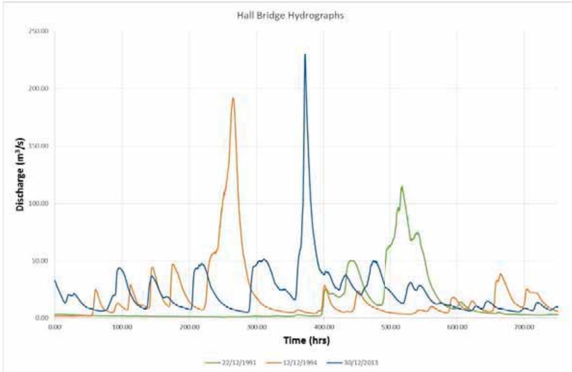
Figure 2-5: Scaled and aligned peaks of hydrographs for the River Nith
