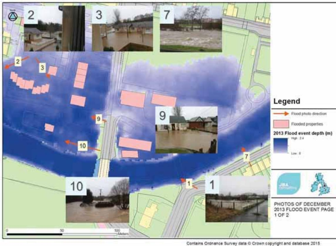
Figure 3-8 December 2013 simulated flood extent with flood photos of the event. Figure 2 of 2. (Photographs courtesy of <http://kirkconnel.org/>)
