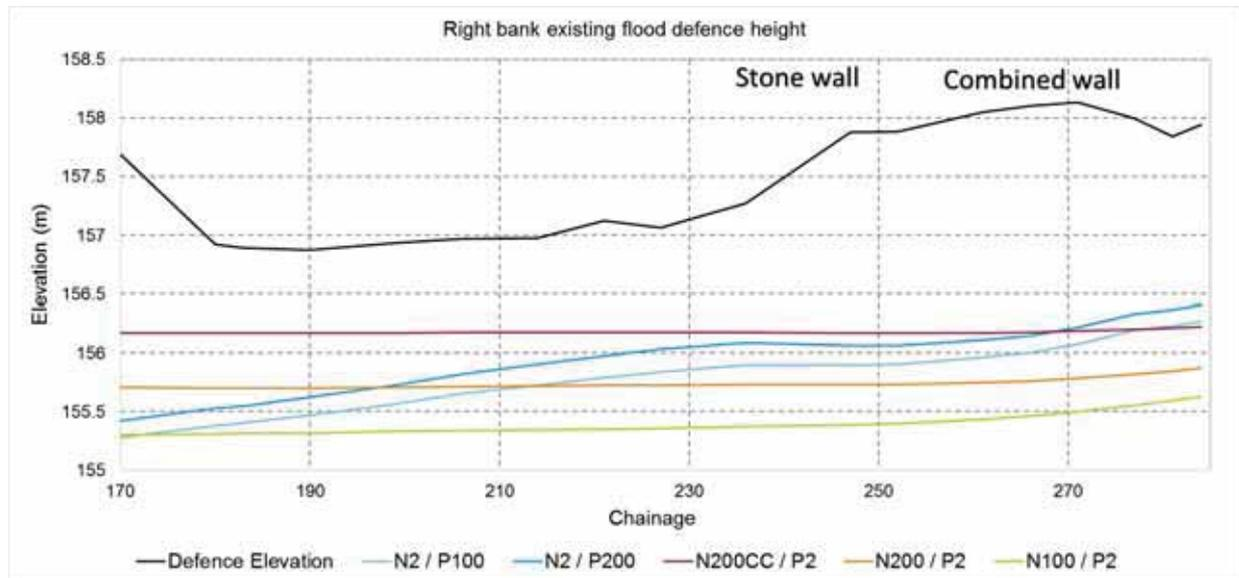
As Figure 4-3 shows there is sufficient freeboard from the top of the defence to the water surface elevation of an extreme event. Freeboard heights based on the 200 year flow event on the Polbower Burn vary from between 1 m and 2.3 m.
