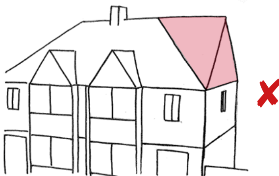
Above: Poorly designed roof extension that unbalances the semi-detached pair
