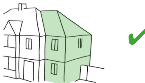
Above: Well designed extensions following the form and pitch of the existing roof.
