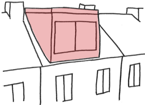
Below: Poorly designed dormers appear excessively large and bulky in the roof
