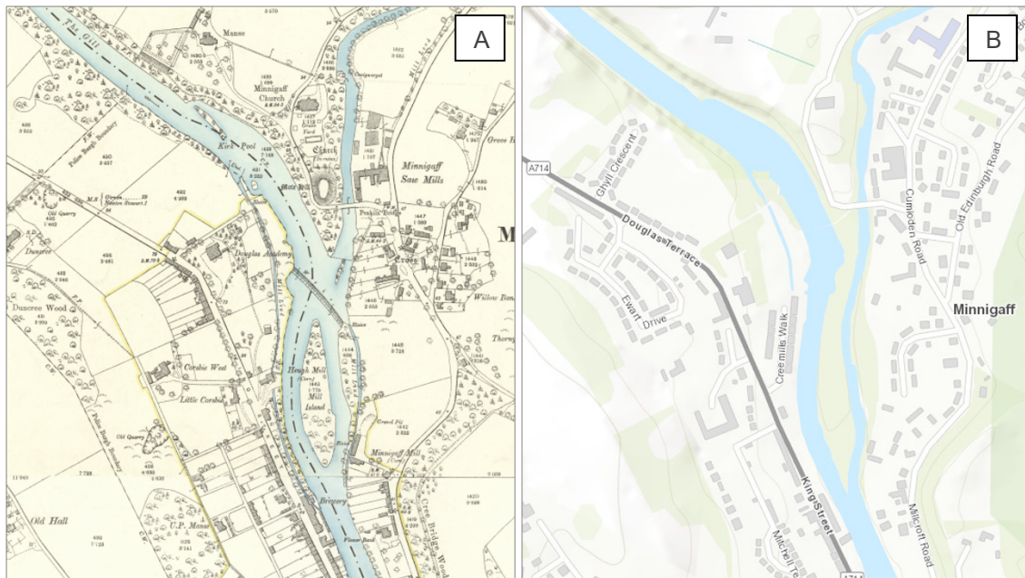
Figure 2.3 Comparison of historical and current OS mapping showing changes in location of the confluence between the River Cree and the Penkiln Burn (A) Historical OS map from 1842-1914 (B) Current OS map.
