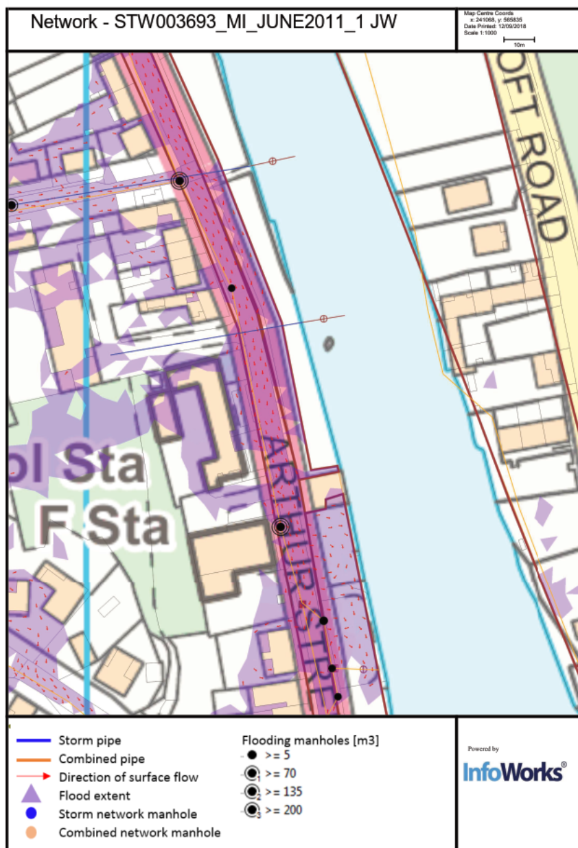
Figure 3.7 Surface water ponding at the Area 11/12 in the post-development situation without mitigation measures.
